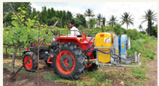
Tractor fitted with electrostatic spray system
